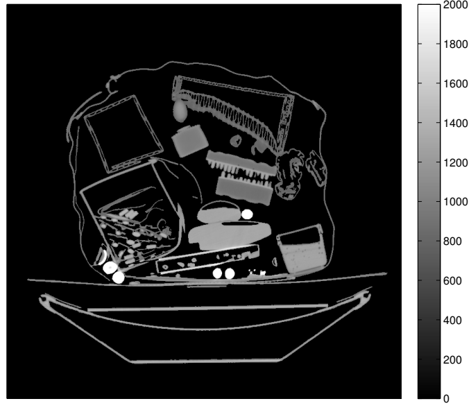
Fig. 4.1. High resolution CT bag scan used as ground truth for the current experiment. Gray scale is in offset Hounsfield units (HU), where Air=0 HU. The original CT image contained reconstruction artifacts due the diversity in composition and morphology of items in the bag, which were removed by masking out the background (set to 0 HU), and retaining only the visible objects. A linear wide-beam projector was then used to generate sinogram data for the current analysis.
