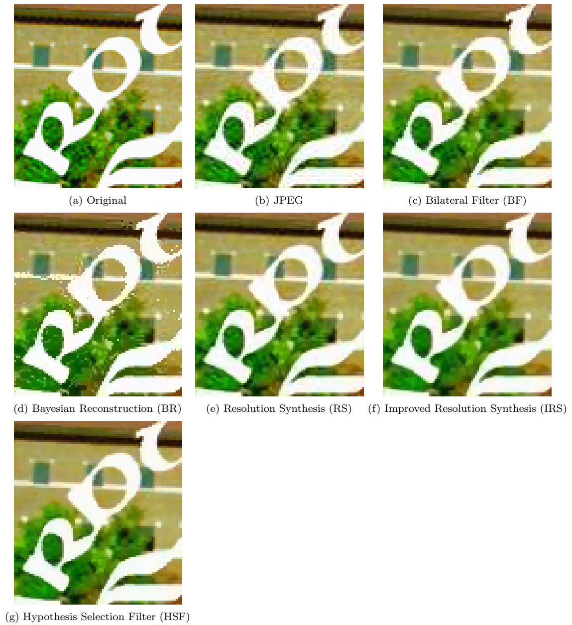
Fig. 2.9. Comparison of decoding results for mixed region 1 (text and natural image) from Image I.
