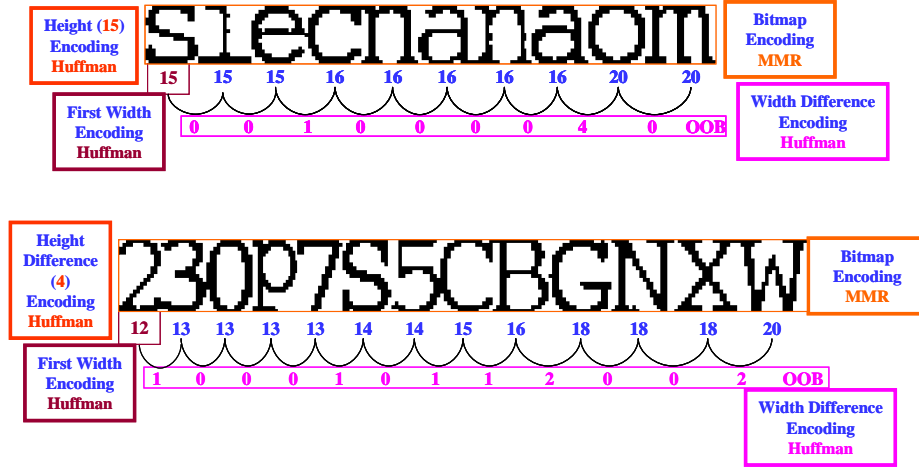
Fig. 1.3. Encoding of a JBIG2 symbol dictionary composed of 23 symbols using Huffman/MMR coding. Dictionary symbols that have the same height are grouped to form a heightclass. Note that the height of the symbols in a heightclass is encoded relative to the height of its previous heightclass. Similarly, the width of a symbol is coded relative to a previously coded symbol in the same heightclass.
