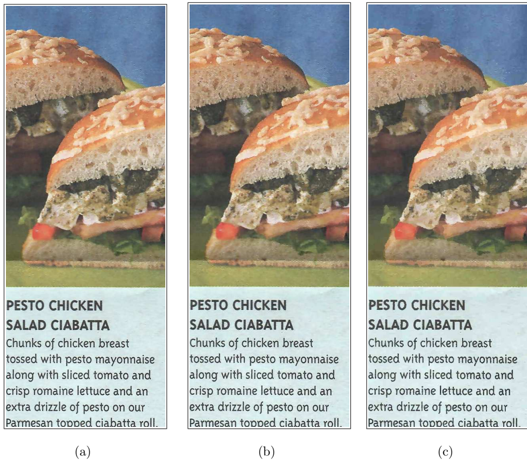
Fig. 2.16. Comparison between images compressed using the JPEG encoder and the MCC encoder. (a) A portion of the original test image “colormix110”. (b) A portion of the reconstructed image compressed with JPEG; achieved bit rate is 0.893 bpp (27:1 compression). (c) A portion of the reconstructed image compressed with MCC; achieved bit rate is 0.491 bpp (49:1 compression).
