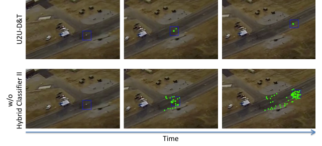
Fig. 12. Results of using Hybrid classifier II during flow point propagation. Blue boxes are the ground truth annotation, green dots are the tracked flow point. First row is the results having Hybrid classifier II to prune flow points and second is the result using optical flow matching directly to propagate the flow points.
