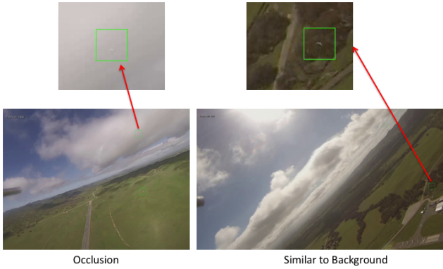
Fig. 1. Challenges in detecting other UAVs: In some cases distant UAVs may be very small and occluded by similar or cluttered backgrounds. In this case, UAVs may not be easily recognizable to human observers.
