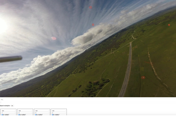
Fig. 6. VATIC Annotation interface: first let annotator initiate object to be annotated and give label and index to the object. Then the software will provide detected object in consequential frames. The Annotator need manually correct the detection.
