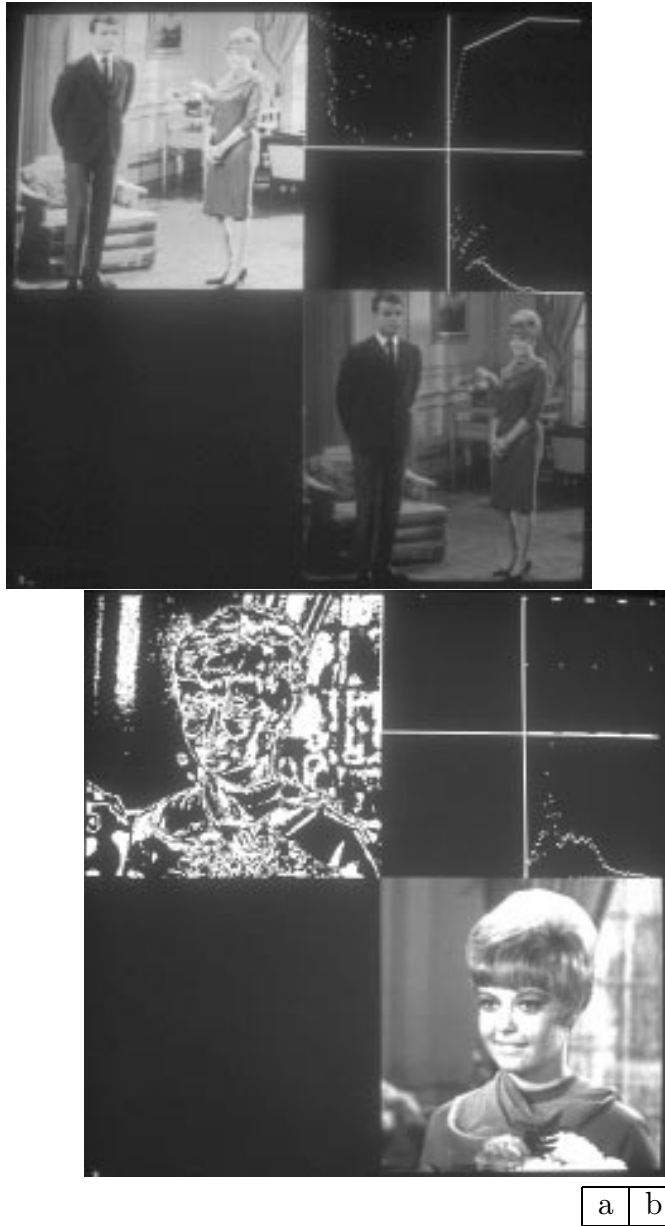
Figure 3: Image brightening and contour generation via gray-scale transformation s .
