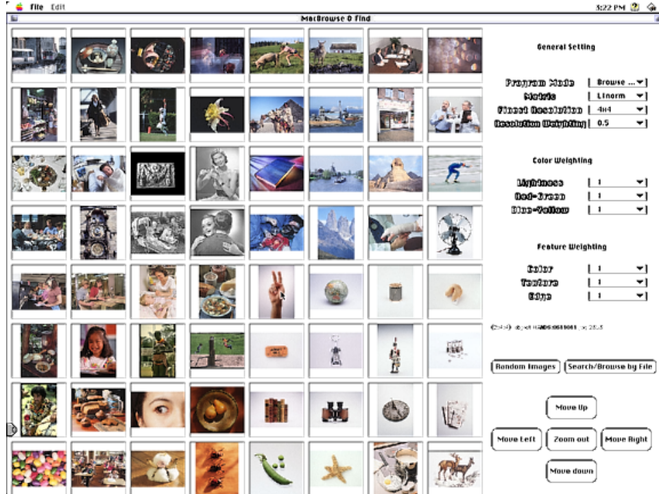
Figure 7. This figure shows the user environment for viewing a similarity pyramid containing 10,000 images. Each image is an icon for a cluster of images. Buttons allow the user to pan across the database, or move up the pyramid. The user can move down the pyramid by “double clicking” on a specific image icon.
