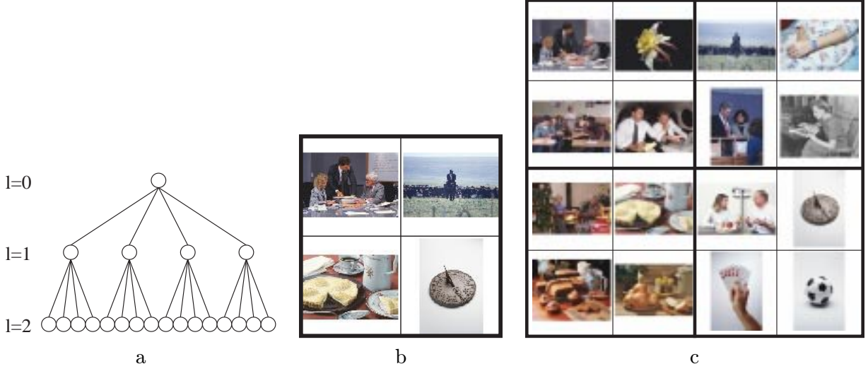
Figure 3. This figure illustrates how nodes are mapped from the quad-tree to the similarity pyramid. There are 24 possible mappings of 4 children nodes to four pyramid nodes. The mapping is chosen to maximize spatial smoothness in image characteristics.
