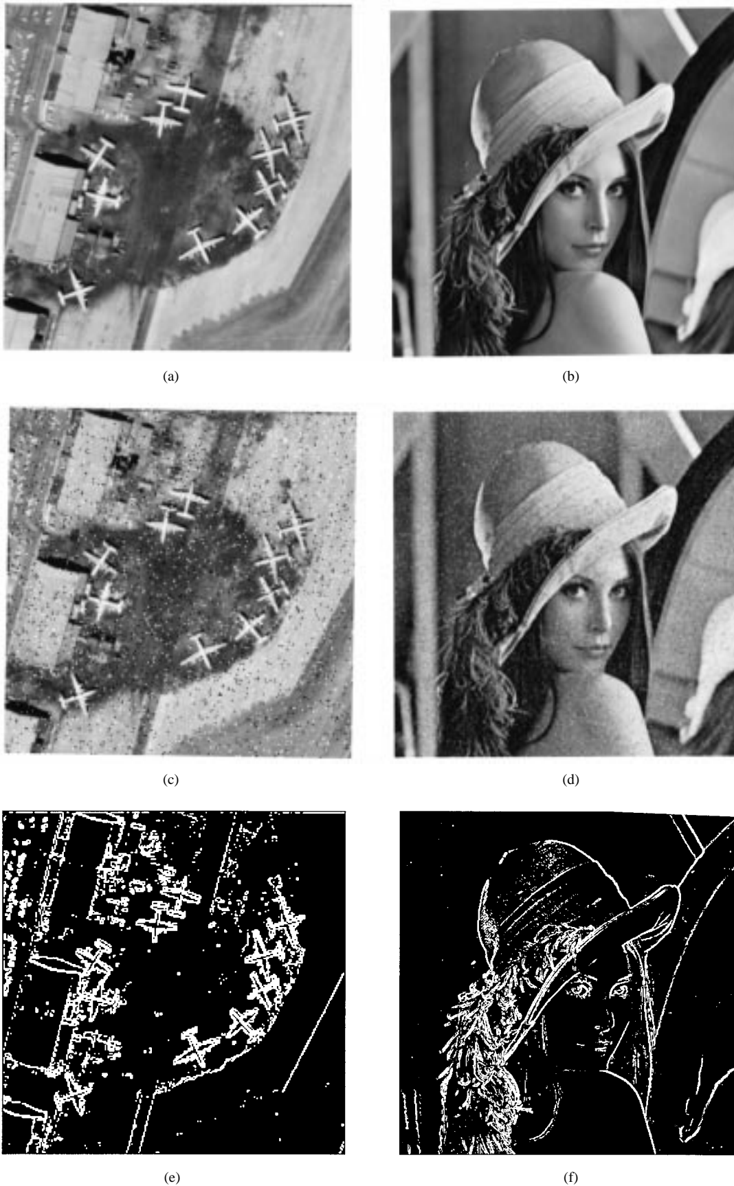
Fig. 7. Test images used in experiments. (a) Aerial photograph with 256 \times 256 resolution. (b) Lenna with 512 \times 512 resolution. (c) Aerial_{I0.05G7.9} . (d) Lenna_{I0.05G7.9} . (e) Reference edge map of (a). (f) Reference edge map of (b). Test images in (c) and (d) are simultaneously corrupted by impulse noise with an occurrence probability of 0.05, and by Gaussian noise with a standard deviation of 7.9.
