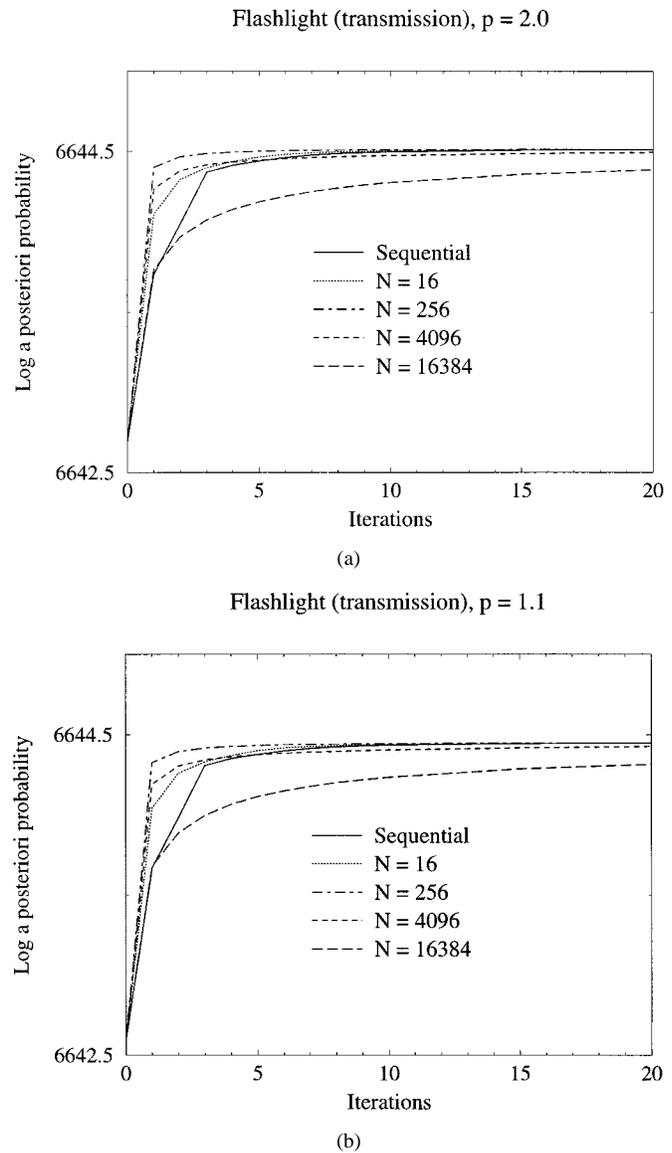
Fig. 13. Convergence of objective function versus iterations for the transmission reconstruction with  $p = 2.0$  and  $p = 1.1$  in GGMRF prior model, employing ICD/FS algorithm in sequential form and varying degrees of parallelism.
