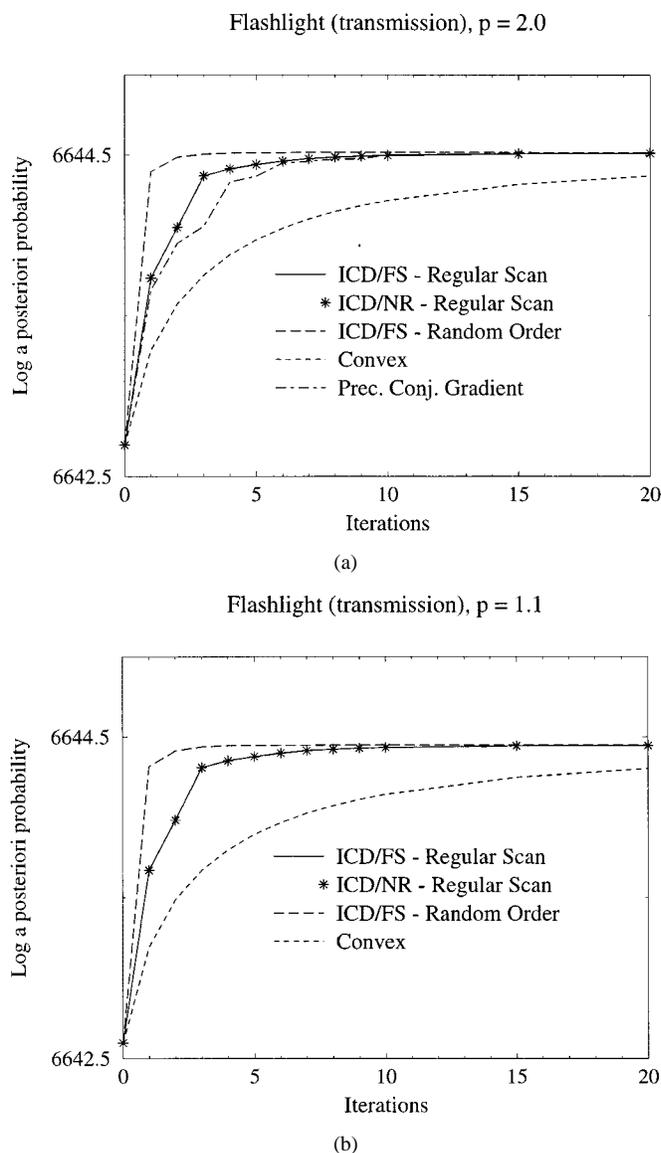
Fig. 8. Convergence of objective function versus iterations for the transmission case with  $p = 2.0$  and  $p = 1.1$  GGMRF prior model, and ICD/FS, ICD/NR, Convex, and (for  $p = 2.0$ ) preconditioned conjugate gradient (PCG) algorithms. ICD/FS is included with both regular and random scan patterns.
