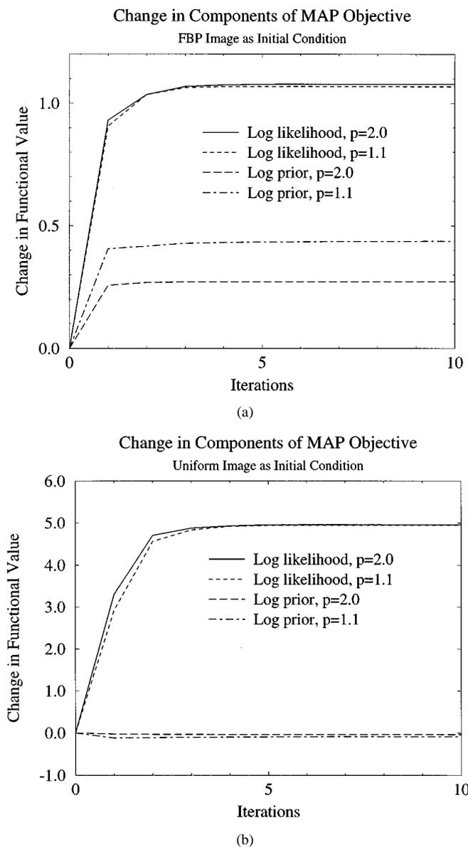
Fig. 7. Gain in  $\log a$  posteriori probability for SPECT case, separated into log-likelihood and log-prior terms of objective function, negatives of which are denoted  $F$  and  $P$  in text. A single iteration includes a sweep across the entire image. (a) Filtered backprojection image as initial condition and (b) uniform image, with total mass equal to that of FBP, as initial condition.
