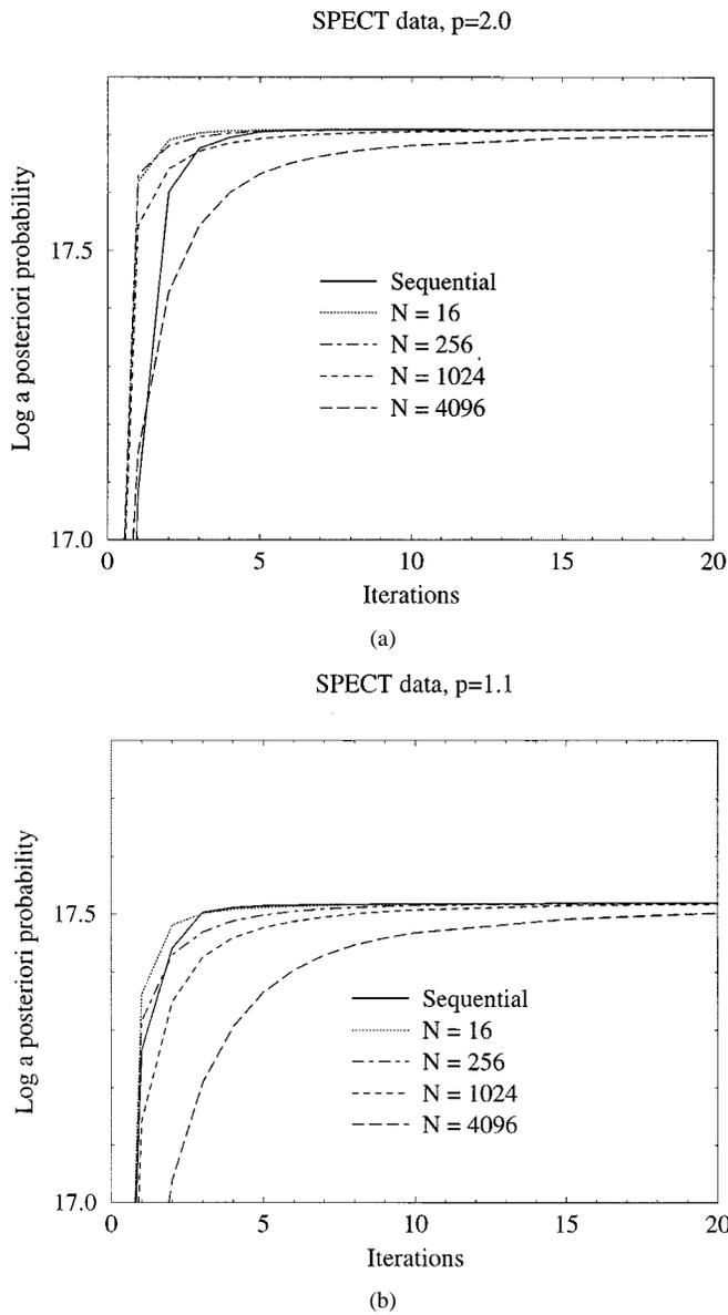
Fig. 12. Convergence of objective function versus iterations for the SPECT heart perfusion data with (a)  $p = 2.0$  and (b)  $p = 1.1$  GGMRF prior model, employing ICD/FS algorithm in sequential form and varying degrees of parallelism.
