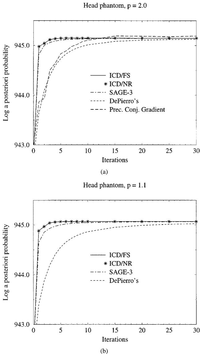
Fig. 5. Convergence of objective function versus iterations for the synthetic head phantom emission case with (a)  $p = 2.0$  and (b)  $p = 1.1$  GGMRF prior models, employing ICD/FS, ICD/NR, SAGE-3, PCG (for  $p = 2.0$ ) and DePierro algorithms. All are initialized with FBP image. Larger values of  $a$  posteriori probability density for PCG are due to violation of nonnegativity constraint.
