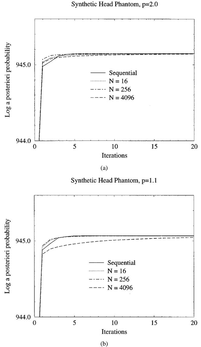
Fig. 11. Convergence of objective function versus iterations for the emission head phantom with (a)  $p = 2.0$  and (b)  $p = 1.1$  GGMRF prior model, employing ICD/FS algorithm in sequential form and varying degrees of parallelism. In this and subsequent plots,  $N$  is the number of pixels updated in parallel.
