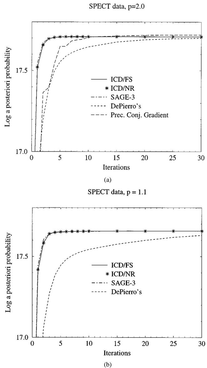
Fig. 6. Convergence of objective function versus iterations for the SPECT cardiac perfusion data with (a)  $p = 2.0$  and (b)  $p = 1.1$  GGMRF prior models, and ICD/FS, ICD/NR, SAGE-3, PCG (for  $p = 2.0$ ) and DePierro algorithms. All were initialized with FBP image except PCG, for which a uniform initialization yielded faster convergence. Higher asymptotic value of objective for PCG is due to violation of nonnegativity constraint.
