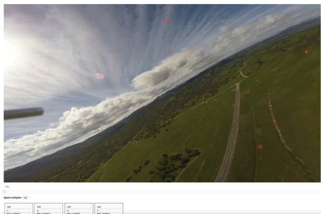
FIGURE 6. VATIC Annotation interface: first let annotator initiate object to be annotated and give label and index to the object. Then the software will provide detected object in consequential frames. The Annotator need manually correct the detection.
