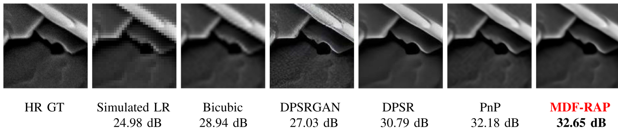
Fig. 5. 4x super-resolution reconstructions of a simulated LR EM image of pentacene crystals with \mu = 0.8 for MDF-RAP. Each shows a zoomed field of view 5.34 \mu wide. MDF-RAP performs well in terms of PSNR (and FRC in Fig. 8) while DPSR produces edges that are even sharper than the edges in the HR GT.
