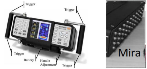
Fig. 15. A picture of the MIRA device used for the experimental data. The device has 10 columns of transducers, where each column acts as a single transducer.
