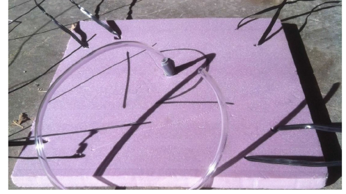
Fig. 14. A picture of defect 12 before embedding it in the specimen, [33]. It is made of dissolving styrofoam.
