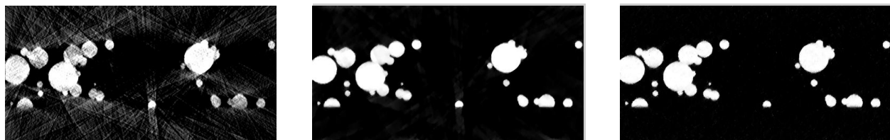
(a) FBP (b) MBIR without Bragg correction (c) MBIR with Bragg correction
