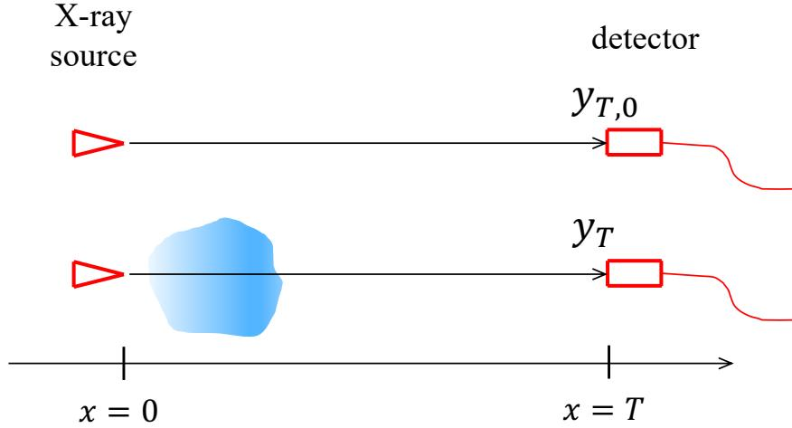
We know that the photon flux,  $y(x)$ , as a function of depth,  $x$ , (units of cm) obeys the following equation
