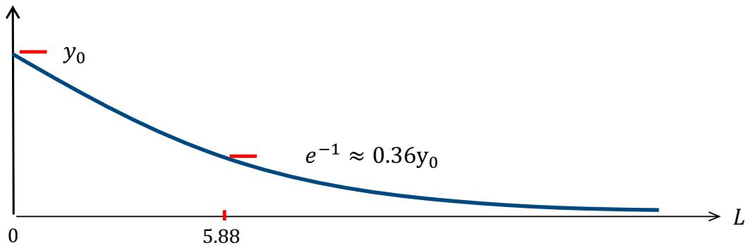
**Problem 4f)** In this problem, assume that the X-ray source energy is at both 40 and 80 keV in equal proportion, so that  $y_0 = 1$  for both cases. Then write an expression the measured  $y_T$  as a function of  $L$ .
