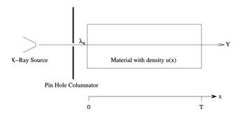
Photons are emitted from an X-ray source and collimated by a pin hole in a lead shield. The collimated X-rays then pass in a straight line through an object of length T with density u(x) where x is the depth into the object measured in units of cm, and u(x) is measured in units of cm<sup>-1</sup>. The expected number of photons at a depth x is given by
