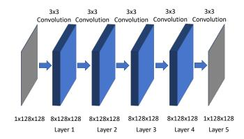
Consider a convolutional neural network (CNN) designed to denoise images as shown in the figure above. The input to the CNN is a noisy image Y and the output is  $\hat{X}$ , an estimate of the noiseless image X. More specifically,
