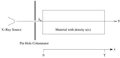
Photons are emitted from an X-ray source and collimated by a pin hole in a lead shield. The collimated X-rays then pass in a straight line through an object of length T with density u(x) where x is the depth into the object measured in units of cm, and  $\mu(x)$  is measured in units of  $cm^{-1}$ . The expected number of photons at a depth x is given by
