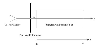
x - depth into material measured in cm
