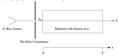
Photons are emitted from an X-ray source and columnated by a pin hole in a lead shield. The columnated X-rays then pass in a straight line through an object of length T with density u(x) where x is the depth into the object. The number of photons in the beam at depth x is denoted by the Poisson random variable  $Y_x$  with  $E[Y_x] = \lambda_x$  where all distances are measured in units of cm and all absorption constants are measured in units of cm<sup>-1</sup>.
