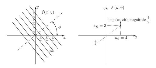
The lines of the plot of f(x,y) represent the locations of the 2D plane wave peaks, which have a magnitude of 1.
