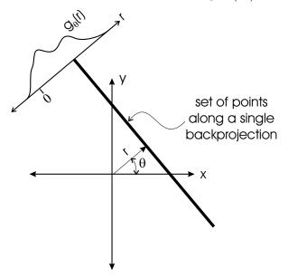
• Complete back projection is formed by integrating (summing) back projections for angles ranging from 0 to  $\pi$ .
