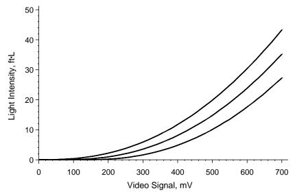
This graph indicates a video signal having a voltage from zero to 700 mV. In a typical eight-bit digital-to-analog converter on a framebuffer card, black is at code zero and white is at code 255.
