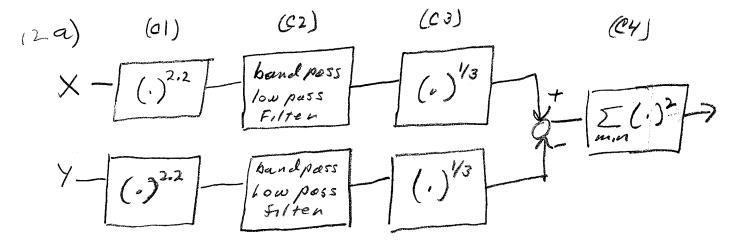
(2 h) (C1) This component convents to linear coordinates, without this component the linear filter would cause tome shifts,
