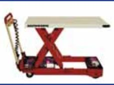
The Backsaver Portable Hydraulic Lift Table is useful for any job that requires lifting, positioning, assembly, stacking/unstacking, transporting, or an adjustable-height work surface. Its 24-inch by 40-inch platform can be raised from 10½ inches to a height of 36½ in 13 seconds by a 12-volt battery-powered motor utilizing low-pressure hydraulics. The device weighs 325 pounds and can lift a 1,100-pound load.
