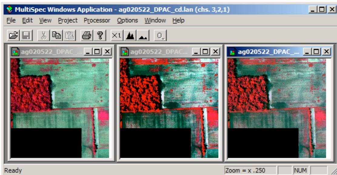
Linear, equal area and Gaussian stretches are illustrated in figure above left to right.
