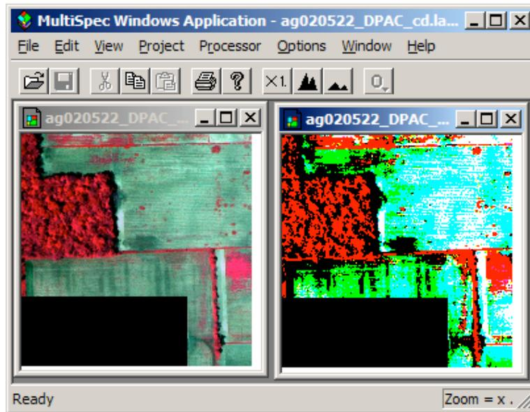
The figure above illustrates 256 display levels per channel (millions of colors) on the left and 2 display levels per channel (8 colors) on the right.
