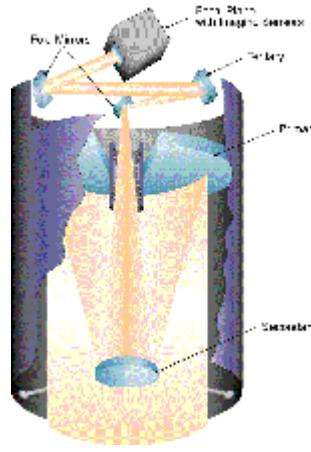
Alignment error of each curved mirror is so small it must be measured in wavelengths of light. "It's equivalent to placing a human hair under one end of a 20-foot plank of wood," says Lloyd. Specifically, the mirrors must not deviate by more than a handful of arc seconds during the rock-and-roll ride into orbit, when settling into zero gravity, across 50° temperature swings inside the spacecraft, or resulting from vibrations caused by spacecraft maneuvering and telescope pointing.
