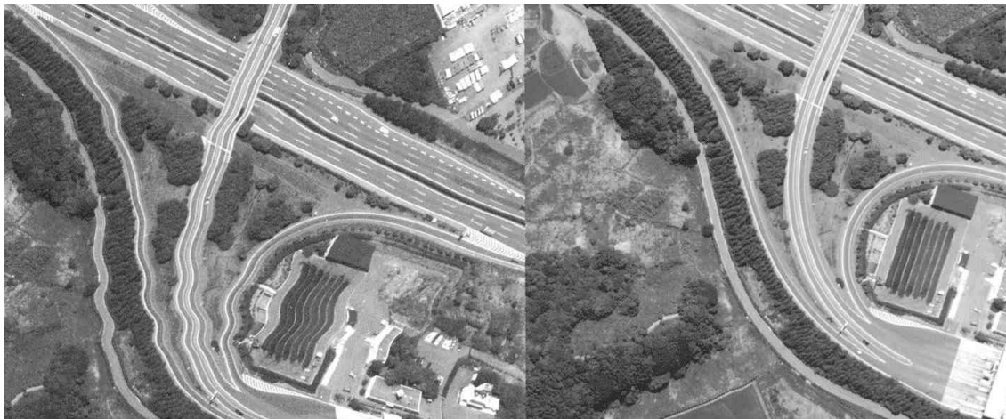
Airborne pushbroom, raw and corrected
