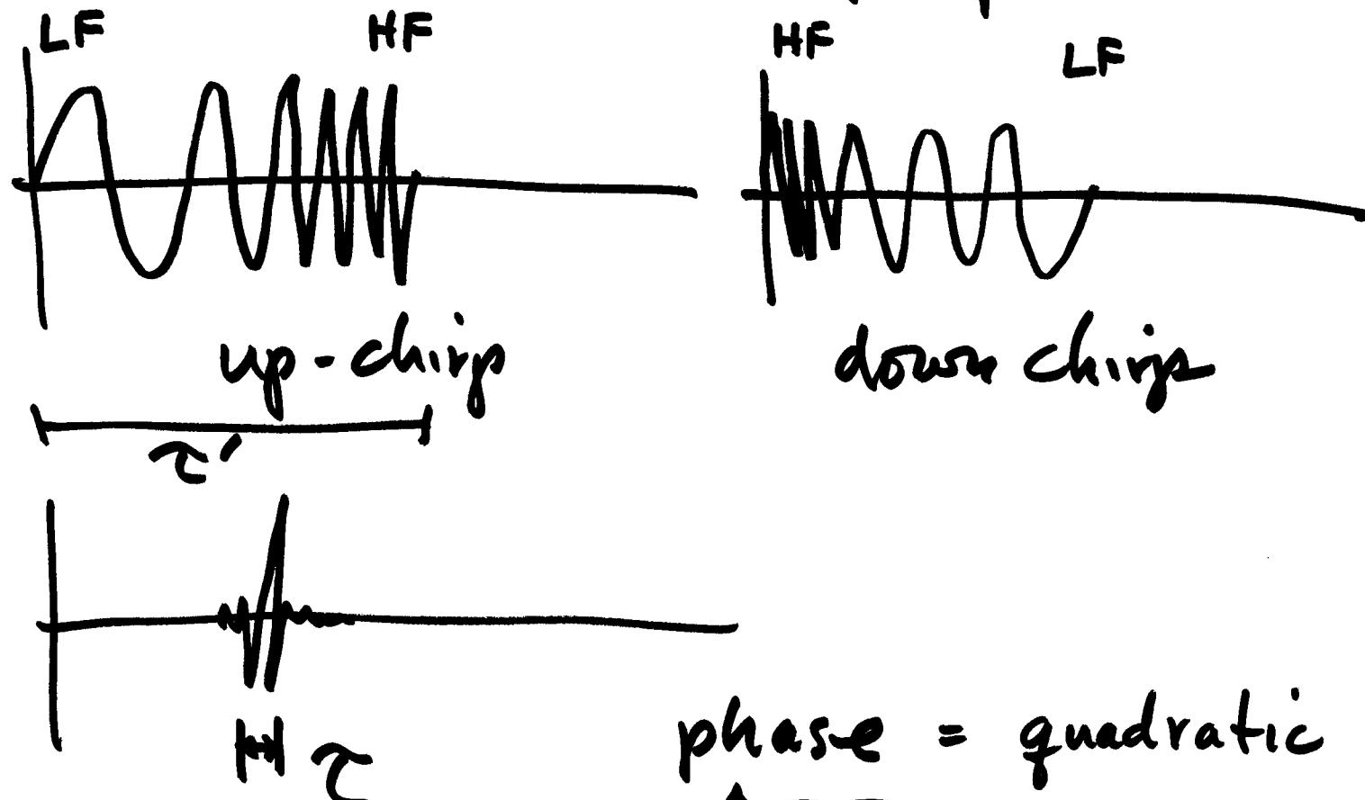
$$A(t) = A \cos \left( \overbrace{\omega_0 t + \underline{\alpha t^2}}^{\text{phase} = \text{quadratic}} \right)$$
