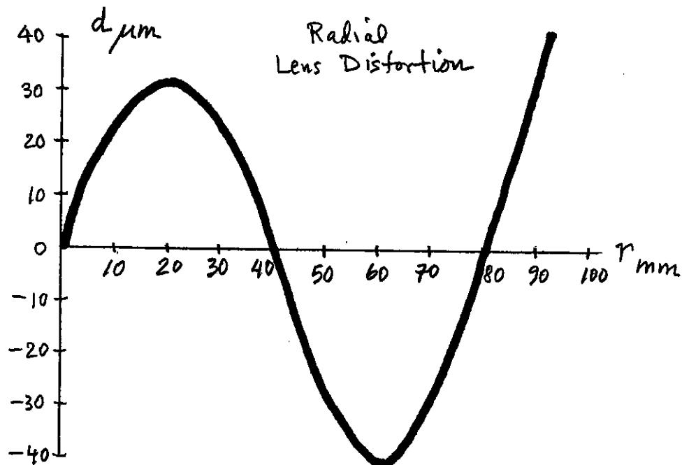
An image point  $(x, y) = (50.000, 33.166) \text{ mm}$  is expressed with respect to the calibrated principal point. Compute the correction for radial lens distortion and apply the correction to the point coordinates.
