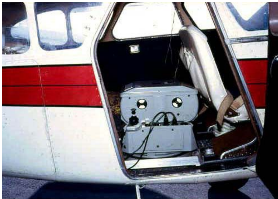
Zeiss RMK in aircraft
