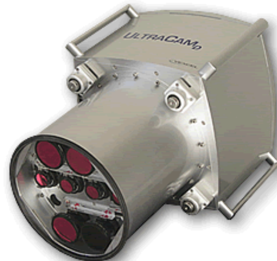
Vexcel UltraCam Digital (note multiple apertures)
