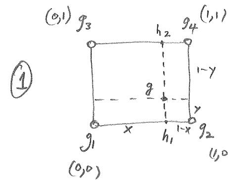
1. linear interp. ( $2 \times$ ) along  $x$ -dir. to produce  $h_1, h_2$
