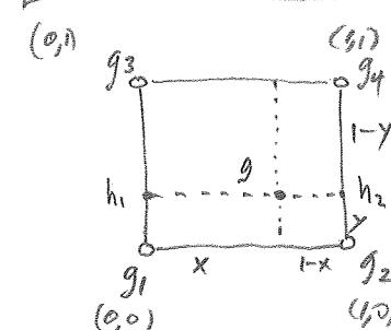
1. linear interp. ( $2 \times$ ) along  $y$ -dir. to produce  $h_1, h_2$
