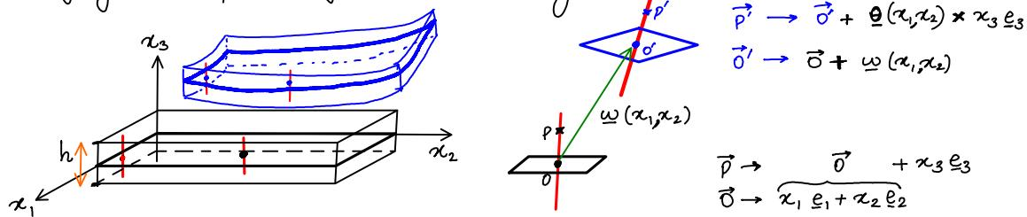
The plate deformation is completely characterized by the deformation of the reference surface ( $\square$ ) and rotation of the rigid fibre ( $|$ ).
