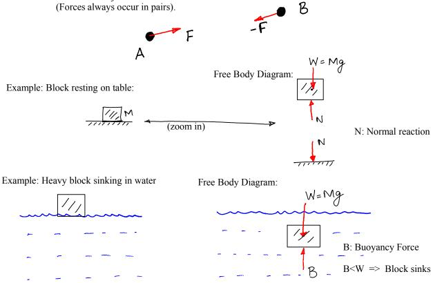
Note: The water is only able to provide a force B to the block, Thus the block is also only able to exert the same force B to the water (and not its full weight W)
