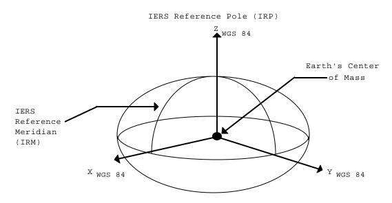
Figure 2.1 The WGS 84 Coordinate System Definition
