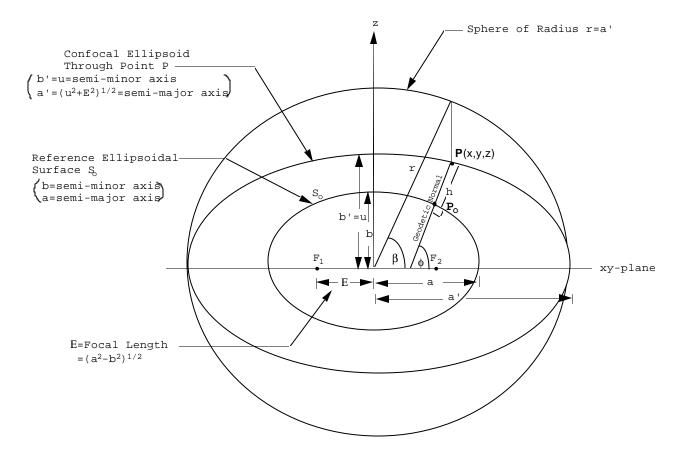
Figure 4.1 Ellipsoidal Coordinates( $\mathfrak{P}$ )
