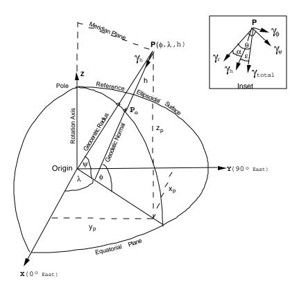
Figure 4.2 Normal Gravity Component  $~\gamma_{\rm h}$
