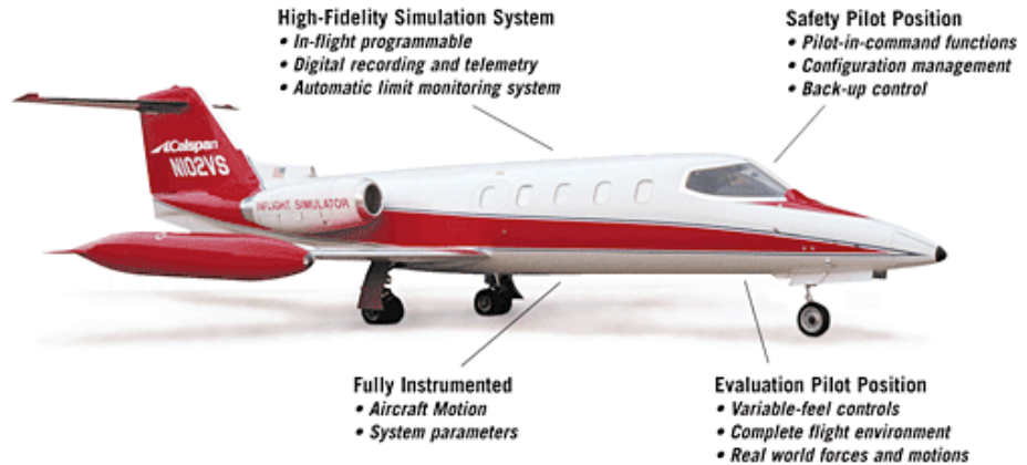
Capabilities of the Calspan's Variable Stability Learjets
