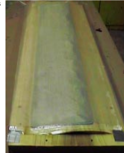
Foam and fiberglass for lower half of wing ready to be vacuum bagged
