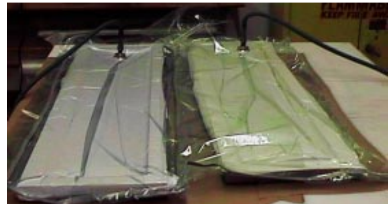
Upper and lower half of a wing in vacuum bags with vacuum applied.
