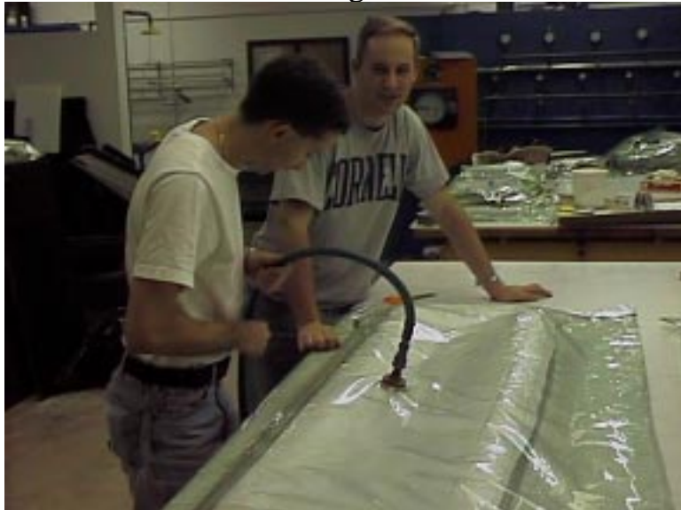
Build-up placed into sealed vacuum bag
