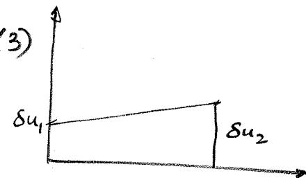
$$\delta \epsilon_x = \frac{\delta u_2 - \delta u_1}{L} \quad \xrightarrow{\text{virtual strain due to virtual disp.}} \text{--- (4)}$$
