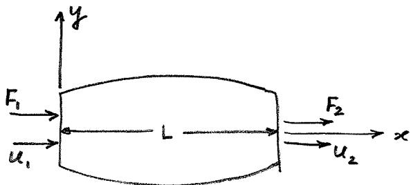
Given: Axial bar of length 'L', constant modulus of elasticity  $E$ ,  $A(x) = A_0 \times \left(1 + \beta \sin \frac{\pi x}{L}\right)$   $\beta$  is known
