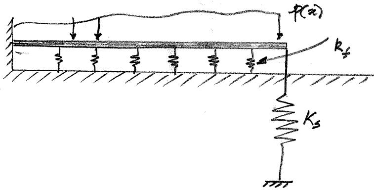
Beam with one end rigidly supported and the other end propped on an elastic spring
