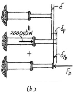
\*4-60. The assembly consists of two posts AD and CF made of A-36 steel and having a cross-sectional area of 1000 mm<sup>2</sup>, and a 2014-T6 aluminum post BE having a cross-sectional area of 1500 mm<sup>2</sup>. If a central load of 400 kN is applied to the rigid cap, determine the normal stress in each post. There is a small gap of 0.1 mm between the post BE and the rigid member ABC.
