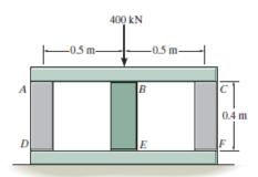
**Equation of Equilibrium.** Due to symmetry,  $\mathbf{F}_{AD} = \mathbf{F}_{CF} = \mathbf{F}$ . Referring to the FBD of the rigid cap, Fig. a,
