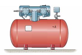
*Hoop Stress for Cylindrical Vessels:* Since  $\frac{r}{t} = \frac{11}{0.25} = 44 > 10$ , then *thin wall* analysis can be used. Applying Eq. 8–1
