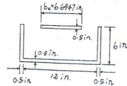
**Maximum Bending Stress :** Applying the flexure formula
