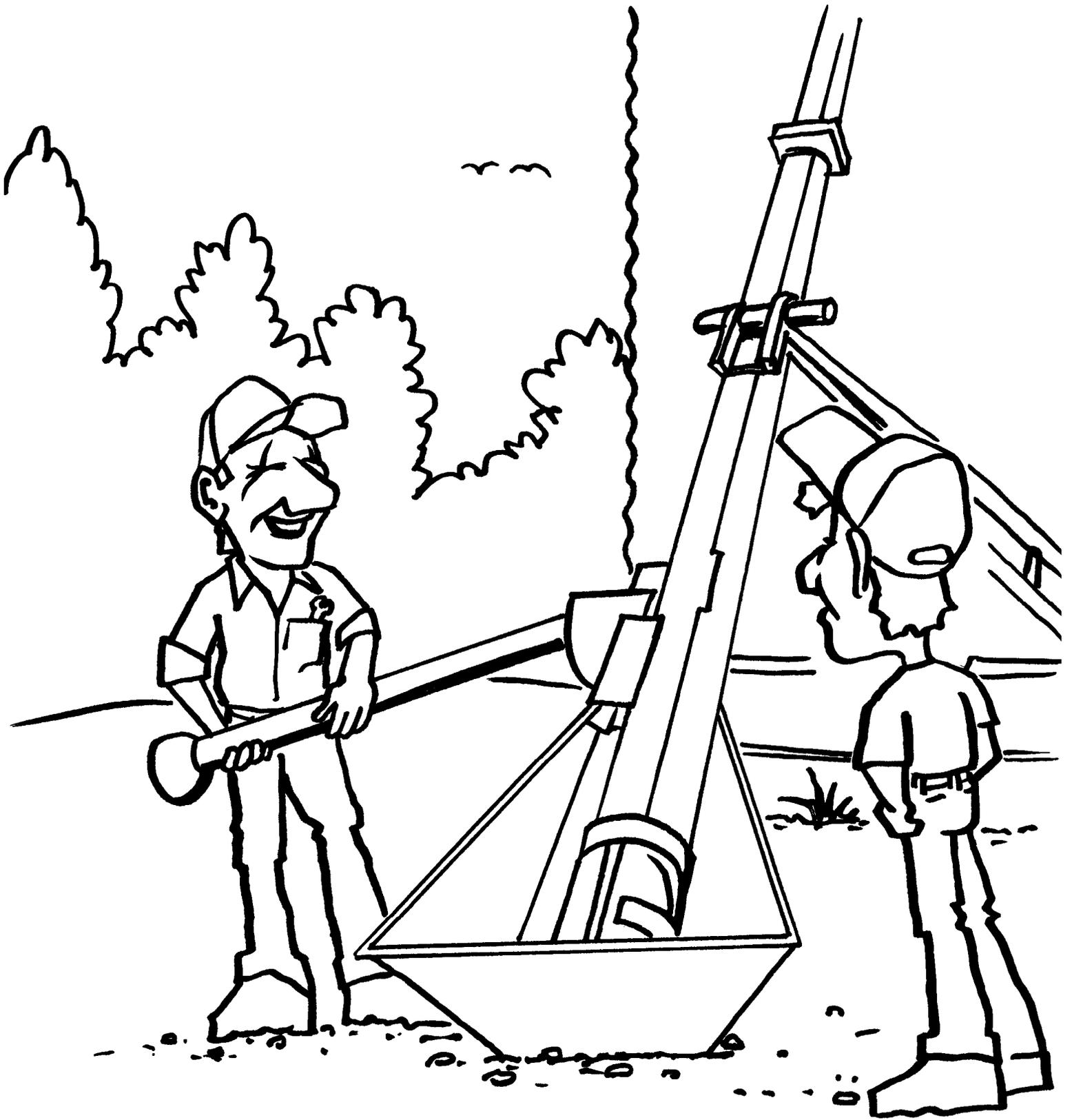
This driveline has an internal stop to prevent it from being extended beyond its safe telescoping limits. As soon as I get out of the way, back up the tractor close enough to the auger to hook it up. Don't forget to lock the brakes and block the wheels before starting the PTO.
