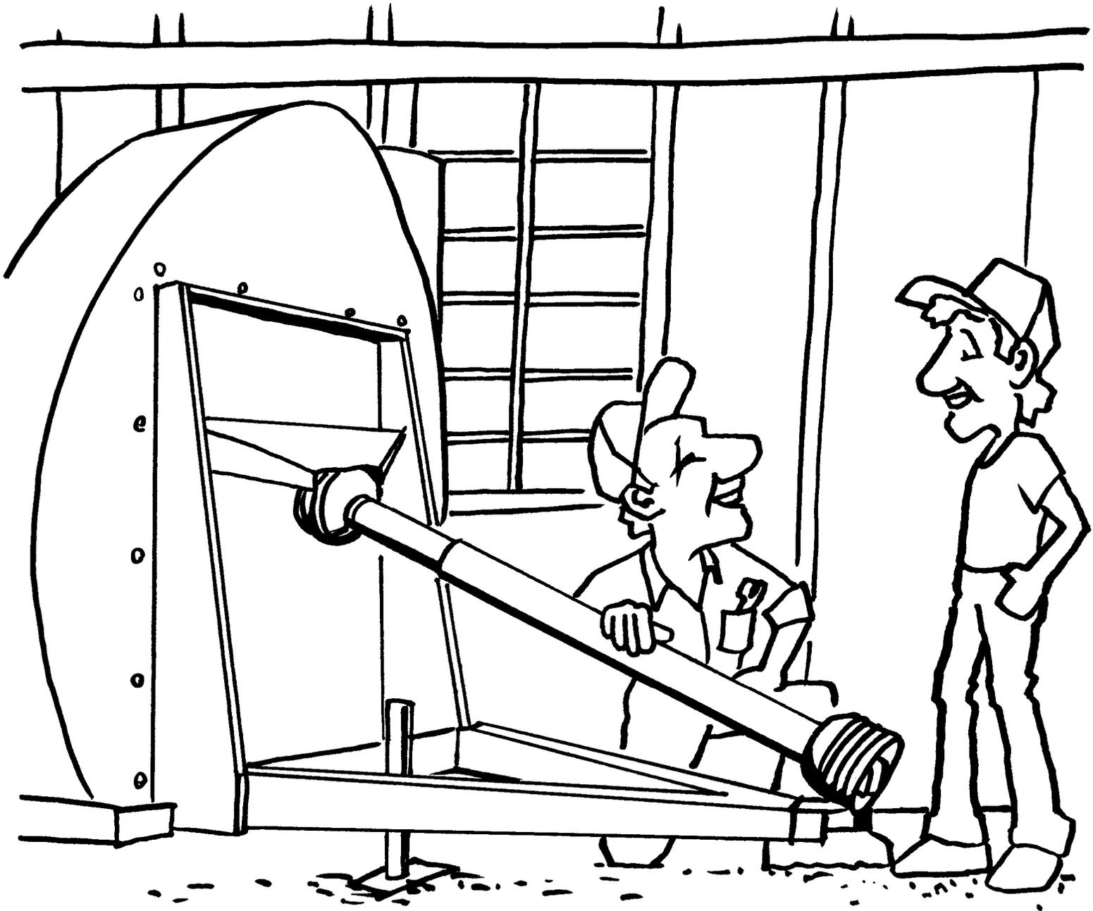
Let's check to insure all guards rotate freely on the shaft, telescope smoothly and that the guard bearings are in good condition. As a last step lubricate the telescoping members, universal joints and guard bearings.
