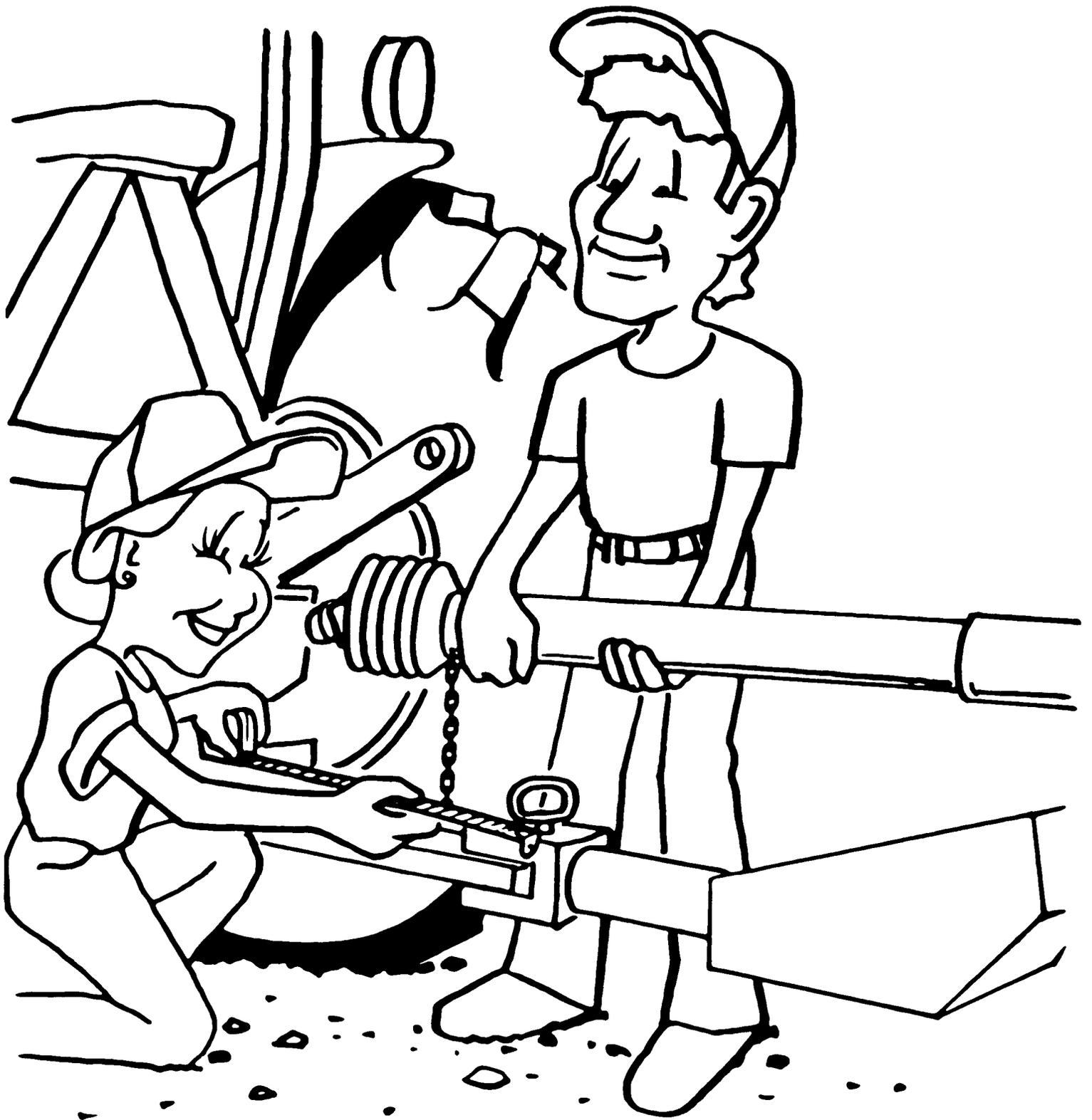
Lets check the draw bar position before we hook up. It has several different locations and if it's not in the right spot the driveline can pull apart or bottom out. Either can result in broken thrown parts.
