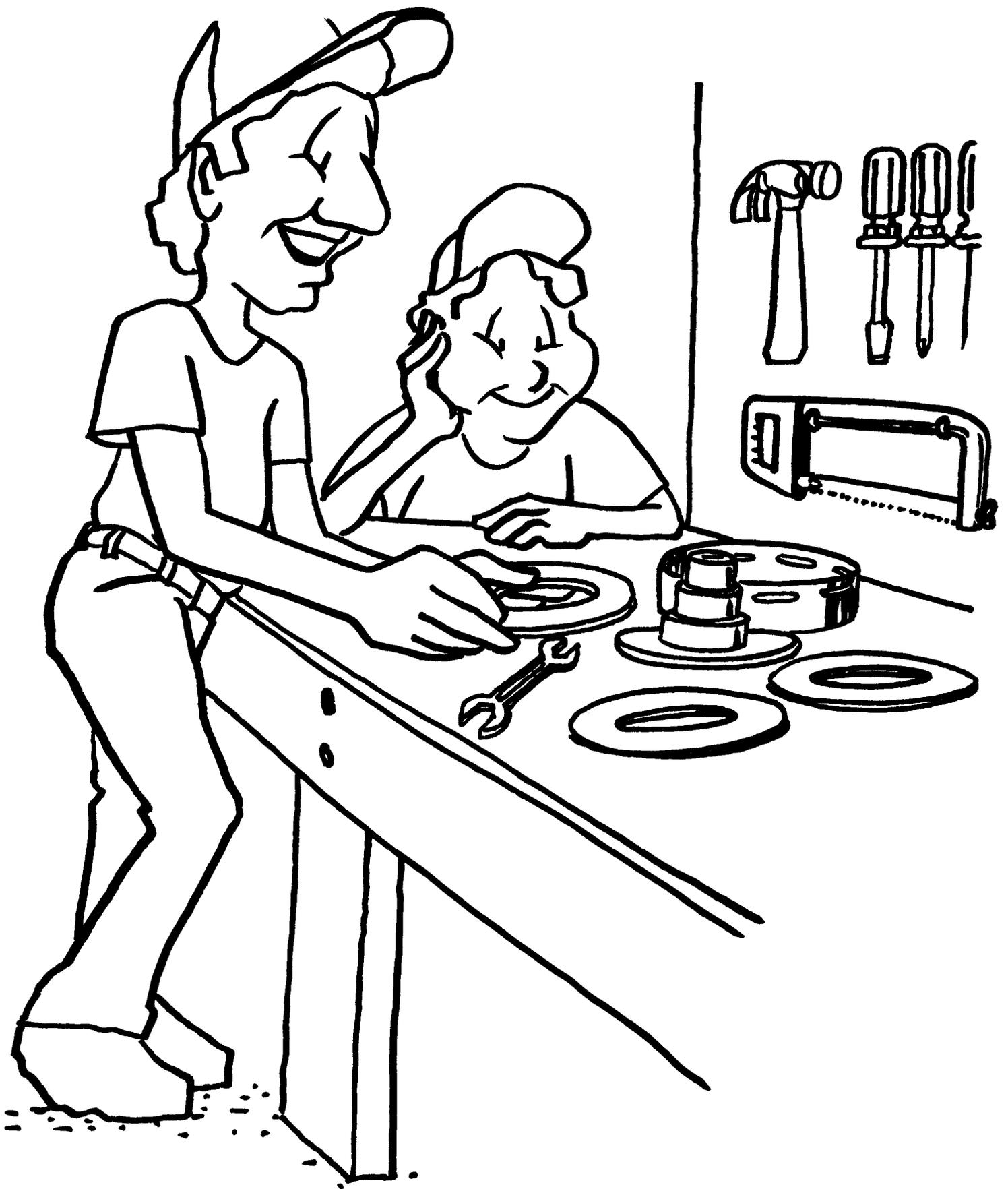
New friction disks will make this safety clutch like new.
