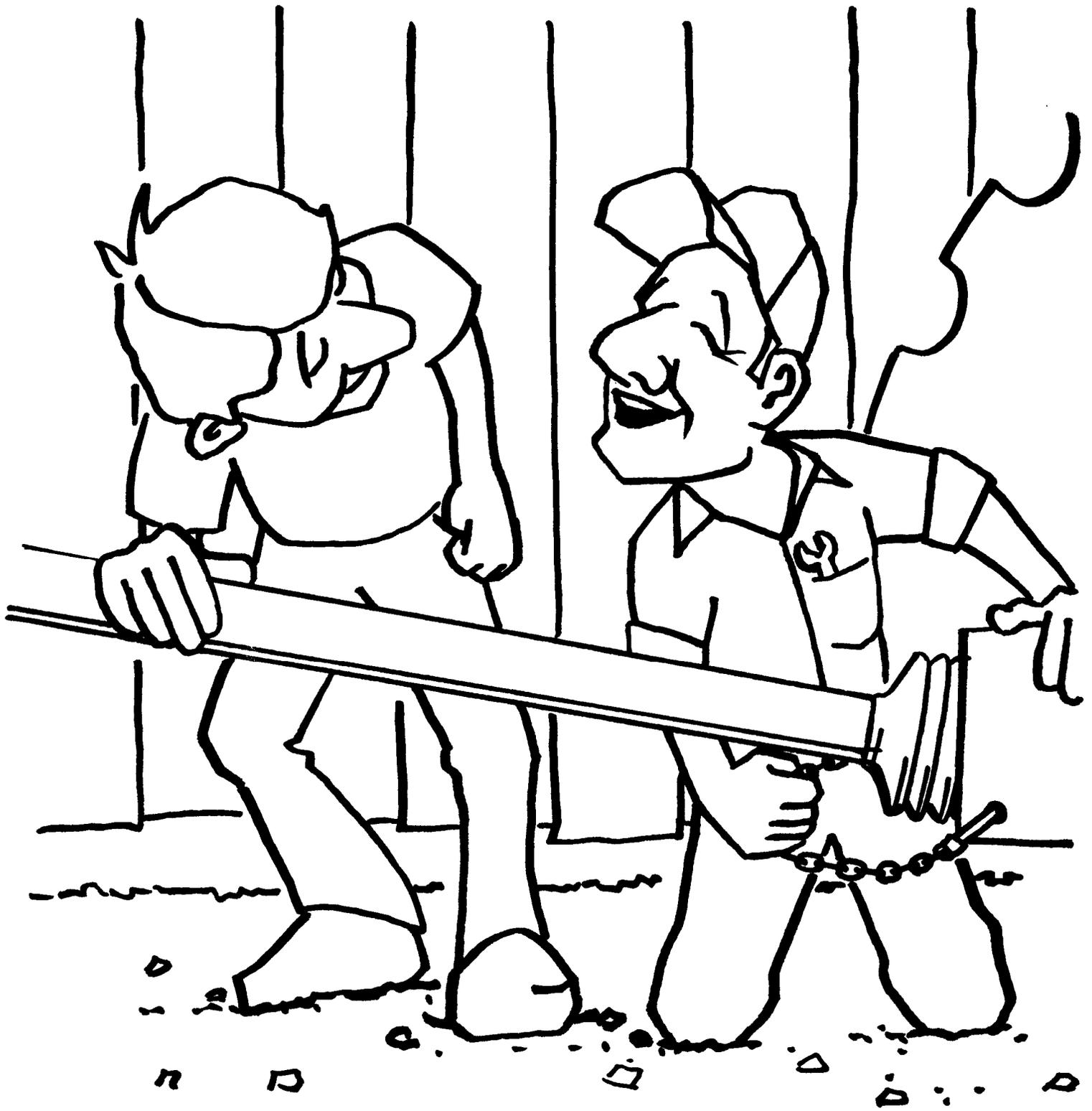
This chain is provided to keep the guard from rotating during operation. Attach it with enough slack to allow for tight cornering.
