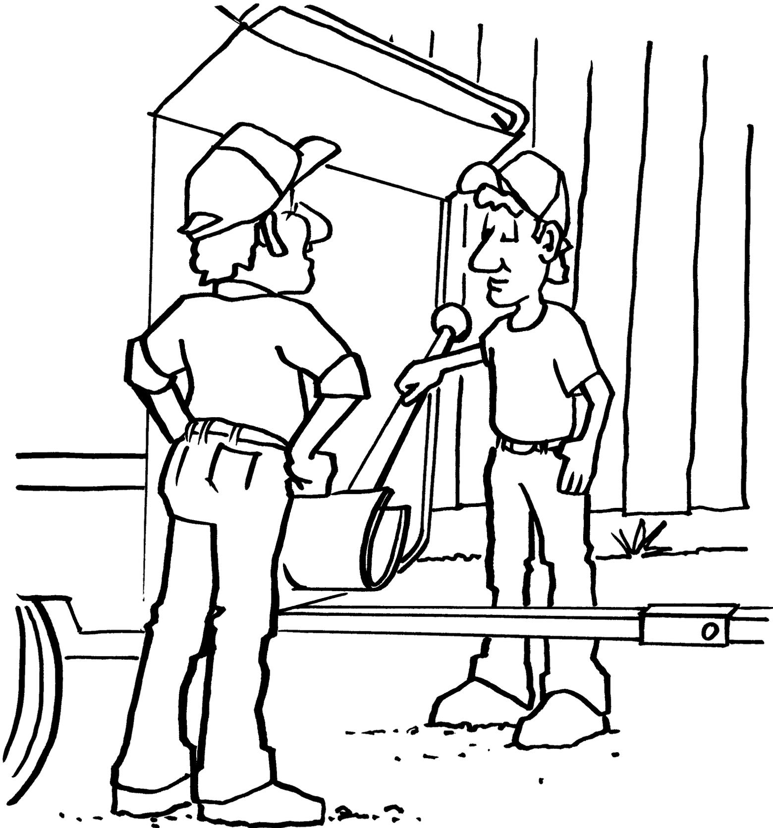
No we can't sway it for the one that needs to be replaced on the grain auger even though it looks like it will fit. Under the guard different strength bars and tubes are used and we might be making a mistake that could cause an injury.
