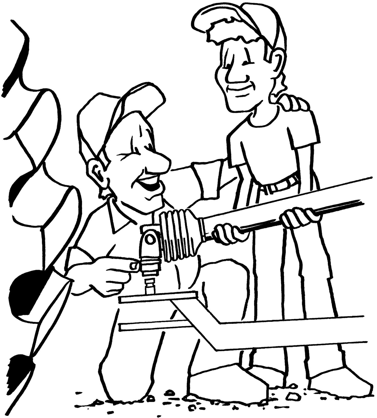
New implements like this one usually have a storage location to keep the driveline up out of the dirt. Always place it in its mount.
