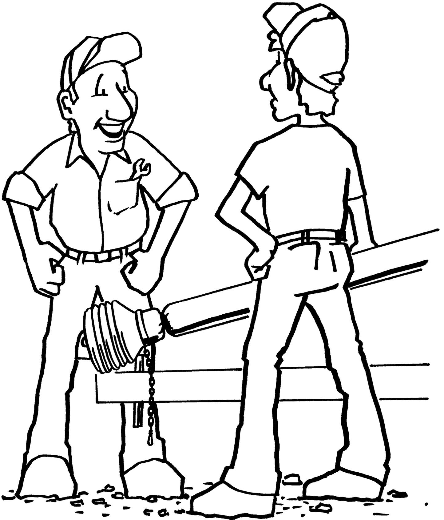
The guard is badly damaged and must be replaced. Go into town and buy a new guard and also some hitch pins with low profile heads so this won't happen again.
