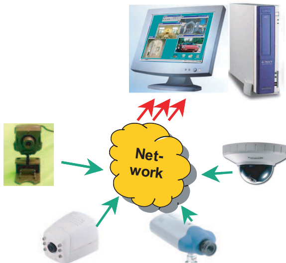
Fig. 1.21. A video surveillance system with distributed cameras.
