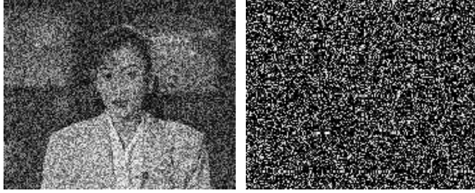
(c) 4LSBs and parity bits are encrypted, (d) 8LSBs and parity bits are encrypted, PSNR=42.25dB. PSNR=9.94dB
