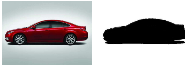
Fig. 3.5. An example of the template extracted from a vehicle belonging to the “sedan” class.
