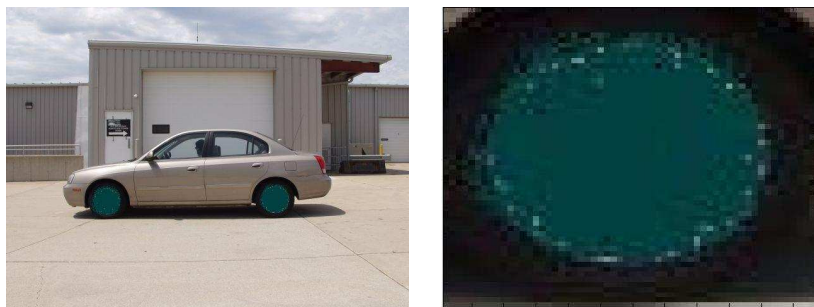
Fig. 4.15. Result of tire extraction on a vehicle with artificially colored dark tires. The position of the lowermost point of the tire was provided as input.
