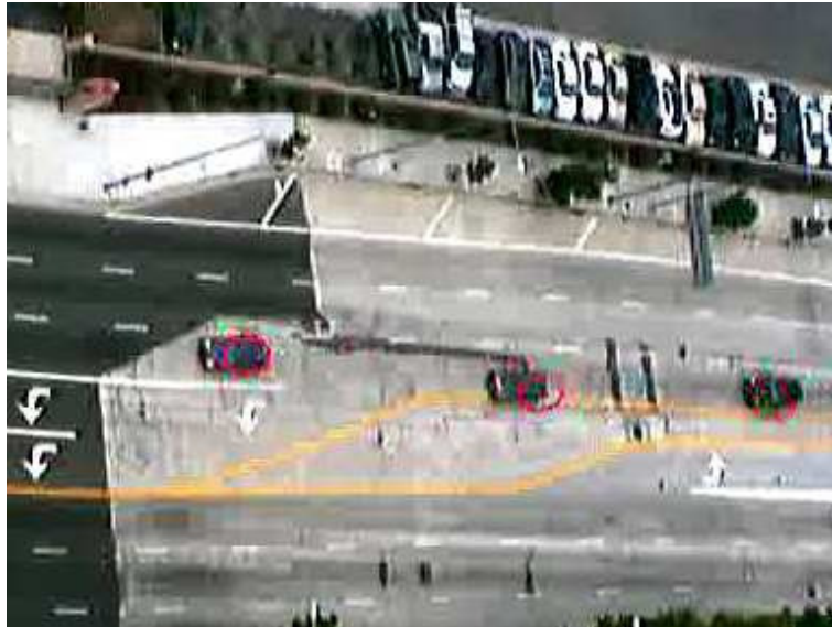
Fig. 4.8. An example of vehicles detected by background subtraction. The image shows a close-up of the scene to illustrate the object ellipses.
