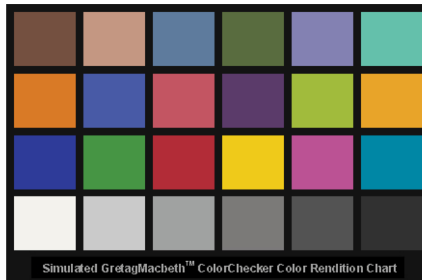
Fig. 3.15. A printed sheet of colored patches used to construct the camera models. Courtesy: Norman Koren [8].
