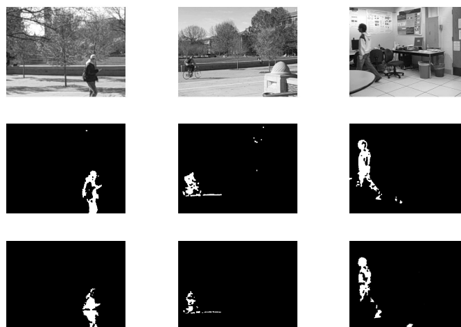
Fig. 4.10. Comparison of MABS (bottom) with GMM (center) for object detection on three test sequences. Columns 1 and 2 show processed frames from sequences with considerable background clutter while column 3 shows a frame shortly after a sudden change of illumination.
