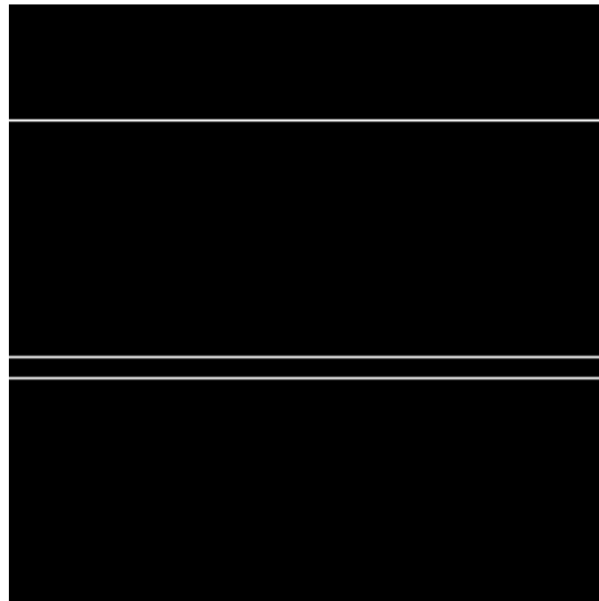
Fig. 5.8. The E-W compass gradient operator detects only edges of the lines in the image shown in Figure 5.7 (a).
