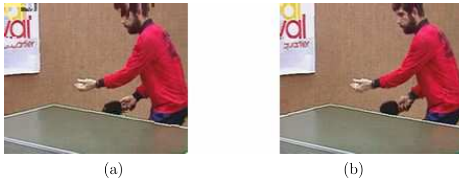
Fig. 2.22. Visual depiction of a frame from the table tennis sequence when 5 packets/frame are lost. (a): Equal Error Protection, WZ rate = 80.19 kbps; H.264/AVC rate=408 kbps; corresponding PSNR=29.11dB). (b) Unequal Error Protection, WZ rate = 71.28 kbps, H.264/AVC rate=408 kbps; corresponding PSNR=35.08dB)
