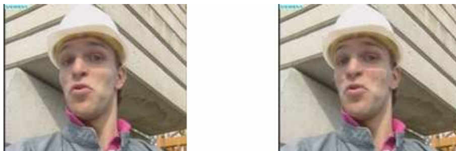
Fig. 4.15. Visual comparison between the original 85th frame (left) and that produced by CAUEP(right: PSNR=38.42dB).
