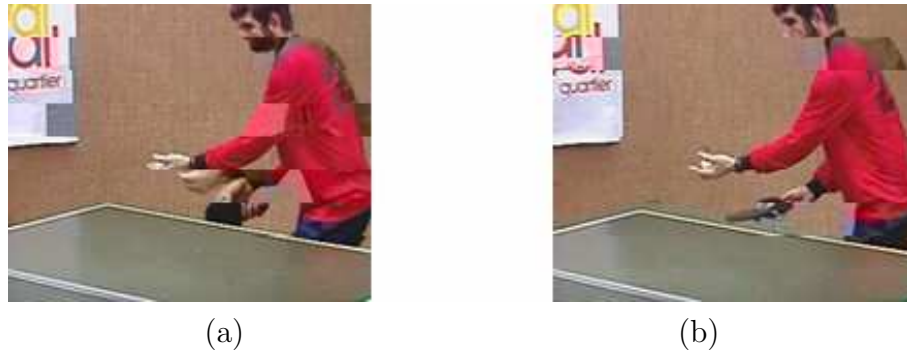
Fig. 2.21. Visual depiction of a frame from the table tennis sequence when 5 packets/frame are lost. (a) Error Concealment performance when the sequence was compressed at a data rate of 479.28 kbps; corresponding PSNR=22.83dB. (b): SLEP with 2 level, parity bit rate WZ rate = 71.28 kbps, H.264/AVC rate = 408 kbps; corresponding PSNR=23.82dB)
