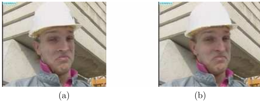
Fig. 2.20. Visual depiction of a frame from the foreman sequence when 4 packets/frame are lost. (a) Equal Error Protection, WZ rate = 80.19 kbps; H.264/AVC rate = 408 kbps; corresponding PSNR = 33.33 dB. (b) Unequal Error Protection, WZ rate = 71.28 kbps, H.264/AVC rate = 408 kbps; corresponding PSNR = 39.55 dB)
