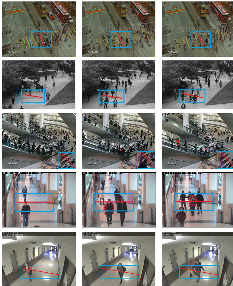
Fig. 4.19. Examples of crowd density estimation on three video sequences. The estimated and true (in parentheses) density levels are (left to right) – Top: 3(3), 1(1), 2(2), Second: 1(1), 3(3), 4(4), Third: 2(2), 3(3), 1(1), Fourth: 1(1), 1(1), 2(2), Bottom: 1(1), 1(1), 1(1).
