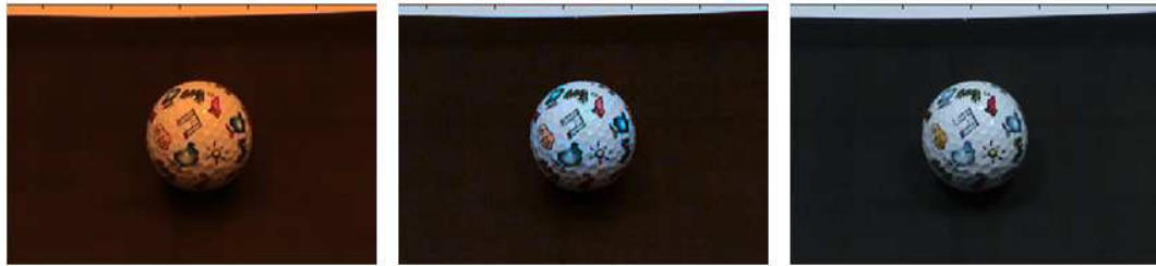
Fig. 5.9. Result of correcting an image with our method assuming known illumination. The columns represent the input image (left), the white corrected image (center), and the image taken under reference conditions (right).
