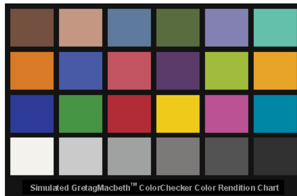
Fig. 5.6. A printed sheet of colored patches used to construct the camera models.
