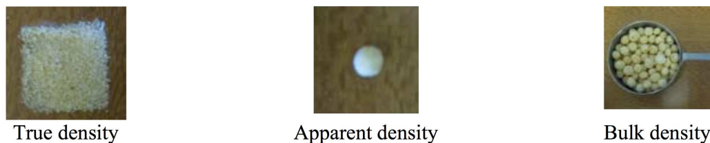
Fig. 3.7. Example of true, apparent and bulk density of the same food (puffed cornflour pellets) (from [31]).
