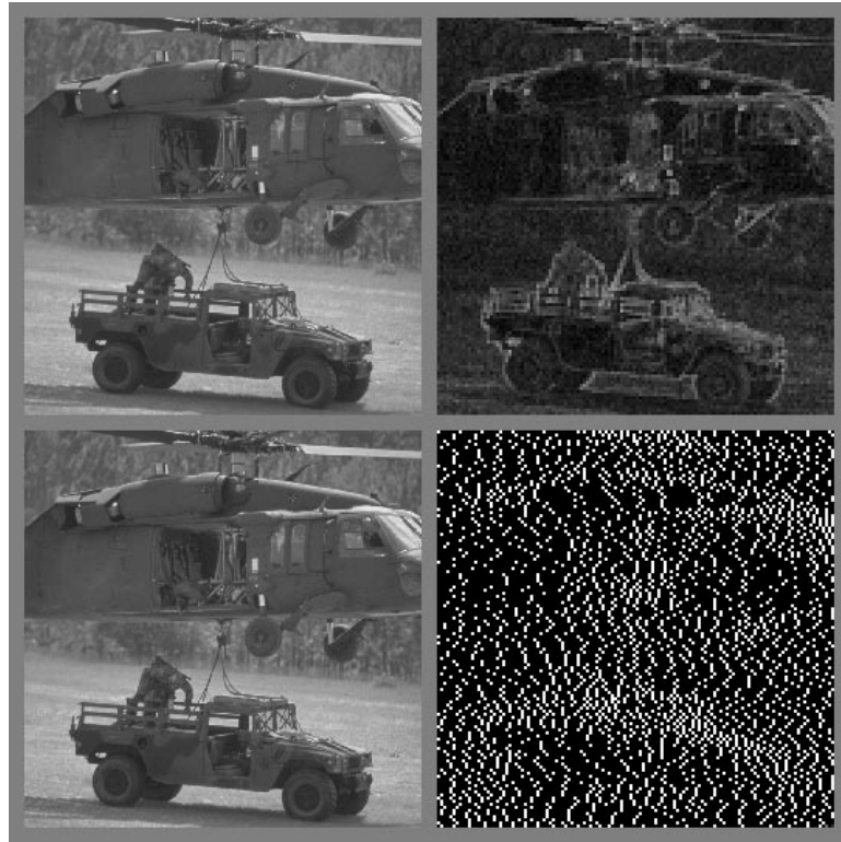
Fig. 3.8. (a) Top left: original 1024 \times 1024 grayscale image. (b) Top right: spatial distribution of the number of bytes in each 8 \times 8 block after Huffman binary encoding. (c) Bottom left: decompressed JPEG image. (d) Bottom right: spatial distribution of the number of bytes in each 8 \times 8 block after output of pipelining realignment algorithm.
