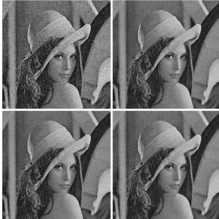
Fig. 5.9. Upper left: noisy version of original image, high spectral correlation; upper right: result of component-wise filter applied in RGB space; lower left: result of filtering only Y in YIQ space; lower right: result of vector filter.
